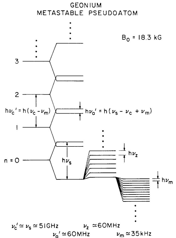
Fig. 4. Energy levels of geonium. Parameter values for an early experiment are shown. They were chosen to make  $\nu_s - \nu_c \approx \nu_z$  for ease of creation of an effective magnetic r.f. field at  $\nu_s - \nu_c$  by shaking the electron at that frequency in the auxiliary magnetic bottle primarily used for the Stern-Gerlach effect [16].
