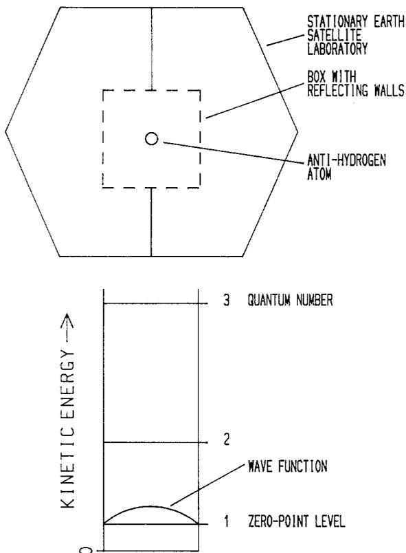
Fig. 2. Individual antihydrogen atom floating at rest in the inertial frame of a stationary earth satellite laboratory [3]. For a box size of  $\frac{1}{2}$  mm the zero-point energy corresponds to a temperature of  $\approx 10^{-11}$  K, and the non-material walls of the box could comfortably be formed by a magnetic trap employing fields no larger than  $100 \mu$ Gauss.
