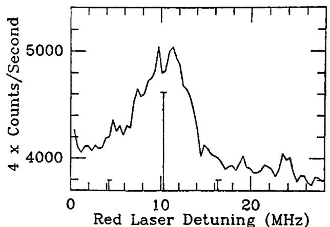
Fig. 16. Doppler shift free optical spectrum of individual Barium ion at  $2.06 \mu\text{m}$  [61]. The absence of side bands at the 6 MHz oscillation frequency, indicates unambiguously, that the oscillation in the trap has an amplitude much smaller than the optical wave length.
