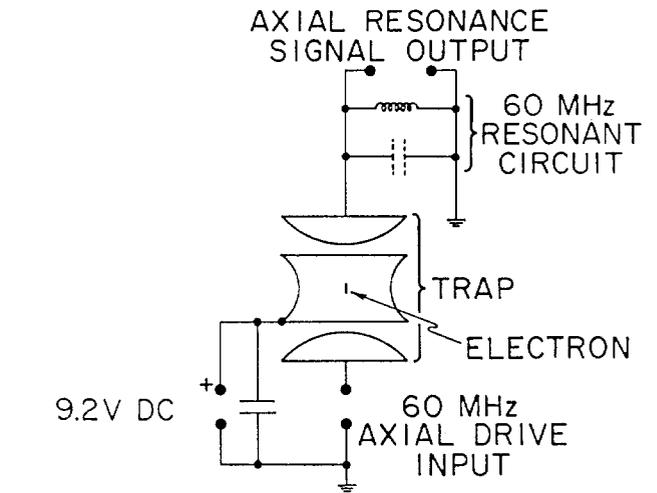
Fig. 11. Trajectory sensor for continuous Stern-Gerlach effect. The spin-dependent parameter of the classical trajectory observed by this axial resonance detector is the frequency of the axial motion  $\nu_z$ .
