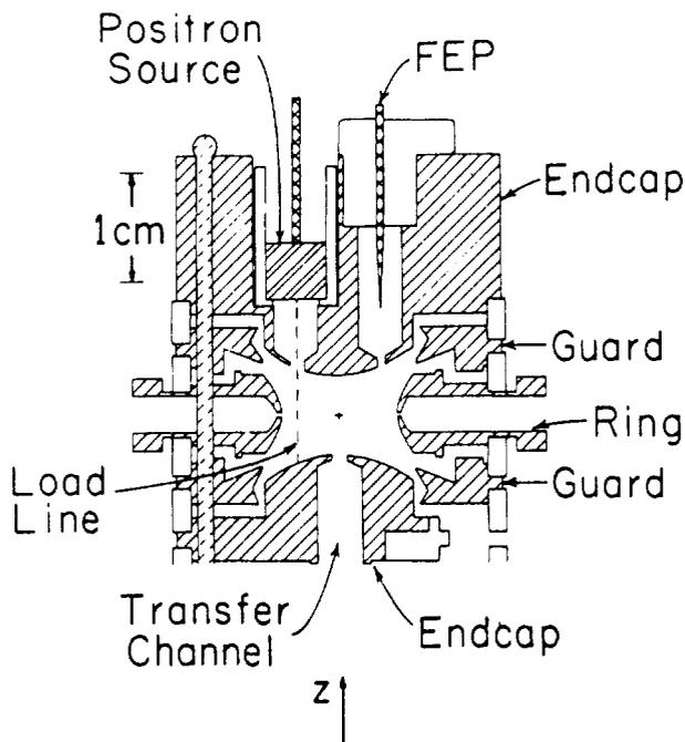
Fig. 15. Auxiliary trap used to catch and store  $\beta^+$  particles from built-in  $< 1$  mCurie source for later transfer into principal trap used for geonium spectroscopy [54].
