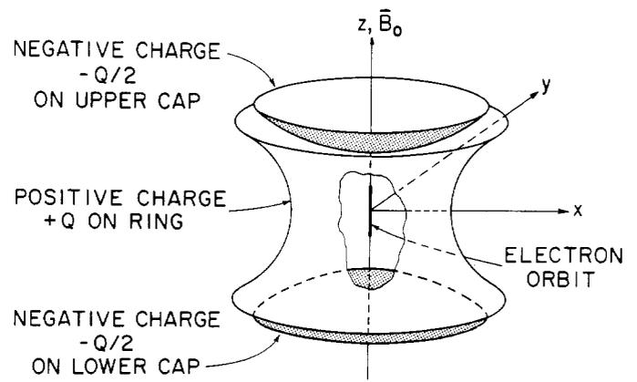
Fig. 3. Geonium atom. The atom consists of an individual electron in the center of a Penning trap [1, 14]. The trap design is related to that of the widely used Penning discharge. The E-field is 0 in the center.
