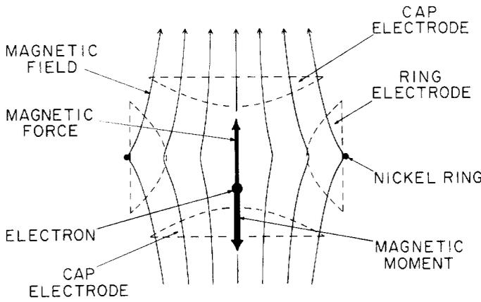
Fig. 10. Shaped magnetic field gradient for Continuous Stern-Gerlach effect. The gradient provides a very shallow supplementary spin-dependent parabolic monitoring potential, slightly shifting the axial frequency  $\nu_z$ . The gradient is created by a ferromagnetic nickel wire wound around the ring electrode, which slightly deforms the principal  $\approx 5$  Tesla field [2].
