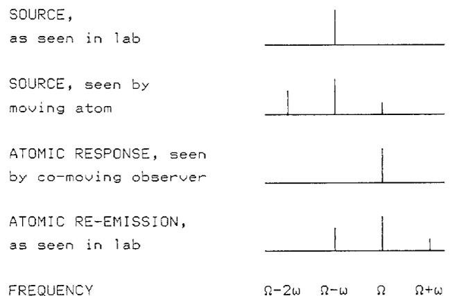
Fig. 7. Side band cooling. The vibrational motion at  $\omega$  of the center of mass of a trapped atom is cooled by a plane wave tuned to the lower Doppler side band at  $\Omega - \omega$  of an internal resonance at  $\Omega$ . In the laboratory frame the source emits photons of energy  $\hbar(\Omega - \omega)$ , which the moving atoms absorbs, and then re-emits with average energy  $\hbar\Omega$ . The balance  $\hbar\omega$  has to come from the vibrational motion which is thereby cooled.
