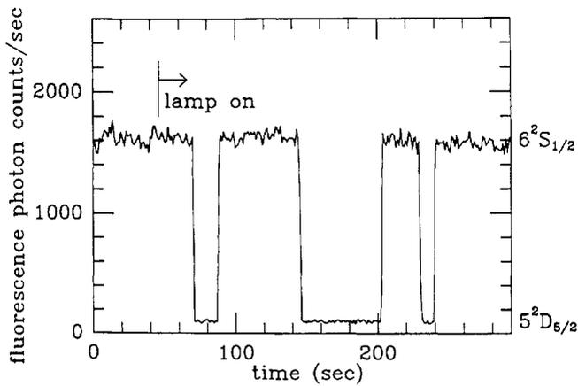
Fig. 17. Demonstration of “shelved (optical) electron amplifier” and quantum jumps. The strong, laser-excited resonance fluorescence is turned off for about 30 s by a jump of the electron into the  $D_{5/2}$  shelf level, causing the loss of  $\approx 10^8$  fluorescence photons [5]. The jump is initiated by the atom absorbing a single photon of lamp radiation!
